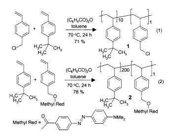
The product copolymer was isolated by solvent precipitation using methanol. In the case of the dye-labeled copolymer 2, this solvent precipitation was quantitative on the basis of the absence of dye label in the supernatant.
